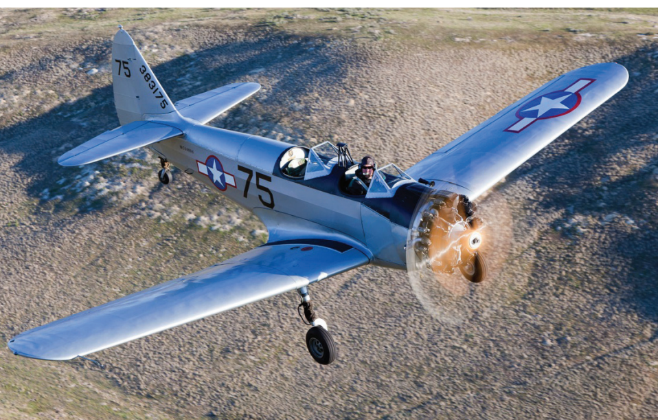
The Fairchild trio of mono-planes was a popular trainer. Each plane had the same airframe but had different engines and cockpits: PT-23, round motor (shown); PT-19, inline Ranger engine and open cockpit; and PT-26, inline Ranger, closed cockpit, and sliding canopy. (Photo by Jim Raeder)
