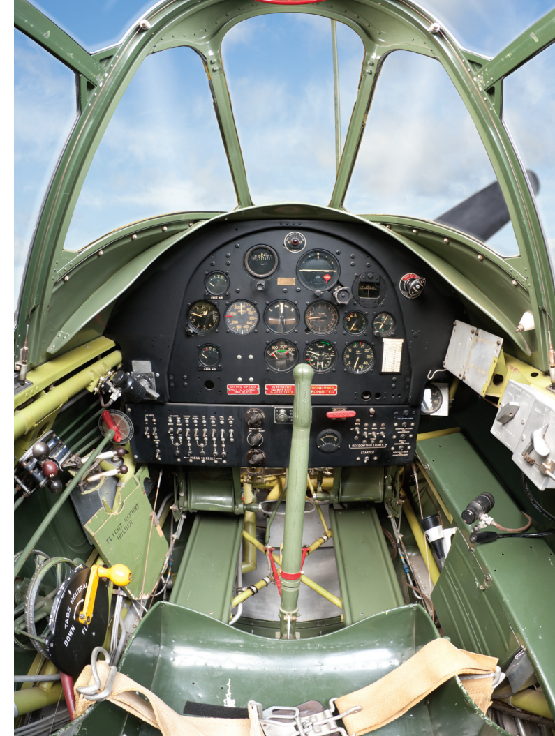
The BT-13’s cockpit was much more sophisticated than that of the Stearman. It was equipped for instrument training. (Photo by Brian Silcox)
