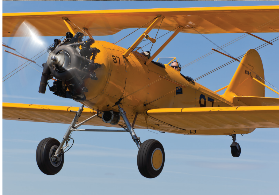
In 1935, the Navy decided that it needed an airplane that it felt fit its training purposes better than the Stearman, so it designed and built the N3N in its own facility. Eventually, the Navy even bought the rights to the R-670 Wright engine and began building its own engines. The design is unique in that, rather than being welded tubes, the fuselage is a triangulated structure using extruded aluminum angles that are bolted together. (Top photo courtesy of Jack Cook; bottom photo by Jim Raeder)
