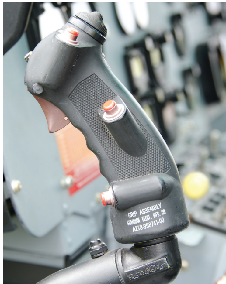
Below, right: From "top hat" to trigger, the stick grip of the Huey had an assortment of buttons and switches. (Photo by Tyson Rininger/EAA)
