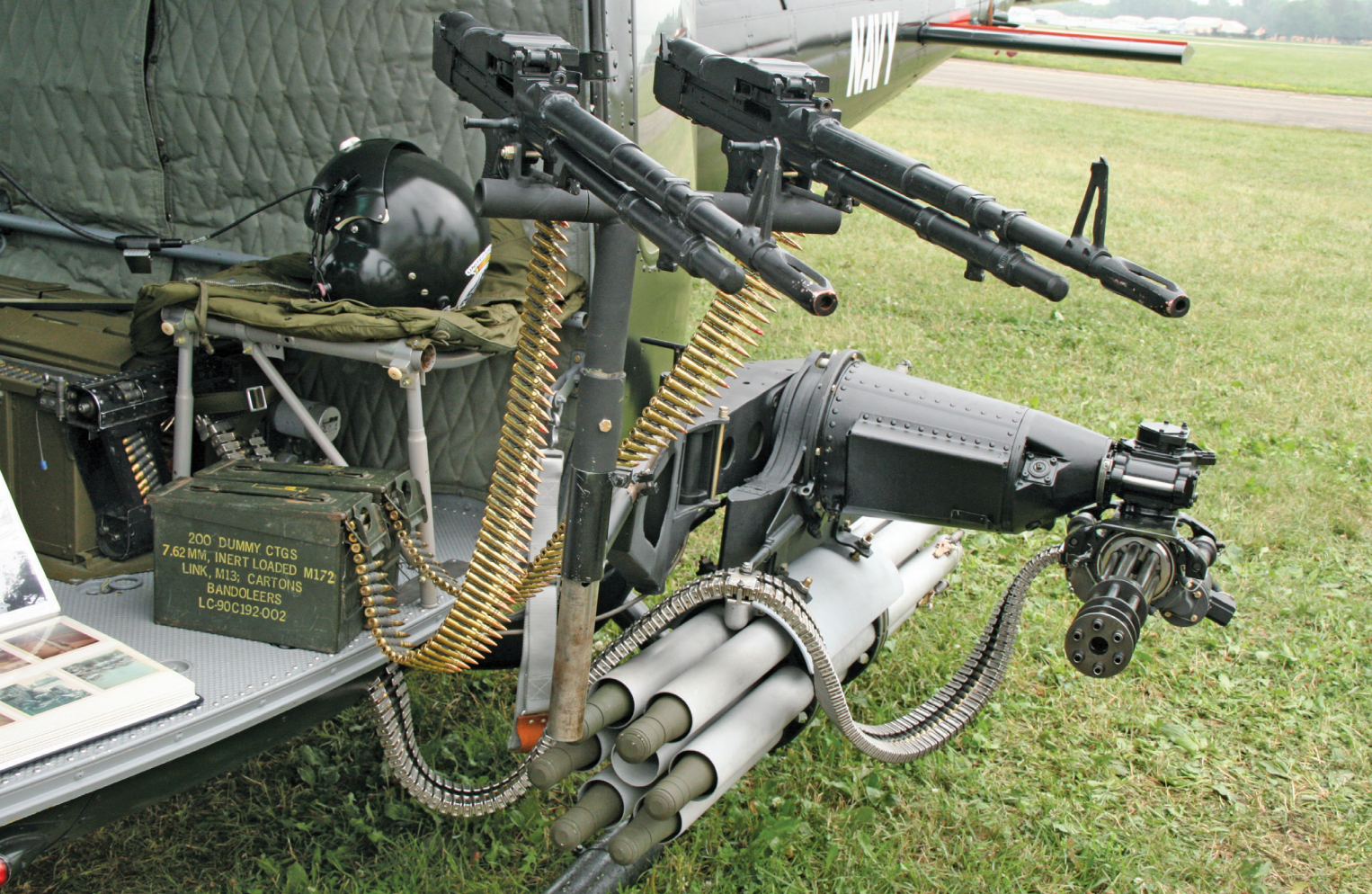
Above: The left side of the Huey was manned by a door gunner who operated dual M-60 7.62 machine guns, while the front-seat pilot operated the M134 7.62 "Mini Gun" and dual 7-shot 2.75-inch rocket pods. (Photo by Dennis Bergstrom/EAA)
