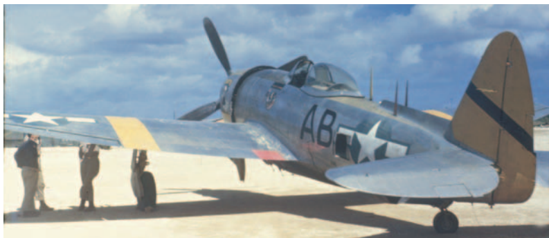
Where the P-47's limited internal fuel capacity and its limited range was a serious disadvantage in the ETO, the P-47N was specifically designed for increased range with a larger wing that held fuel, the first in a Jug. When equipped with drop tanks, the airplane had so much range the pilot became the weak point. (Photo courtesy of Jeff Ethell Archives)
