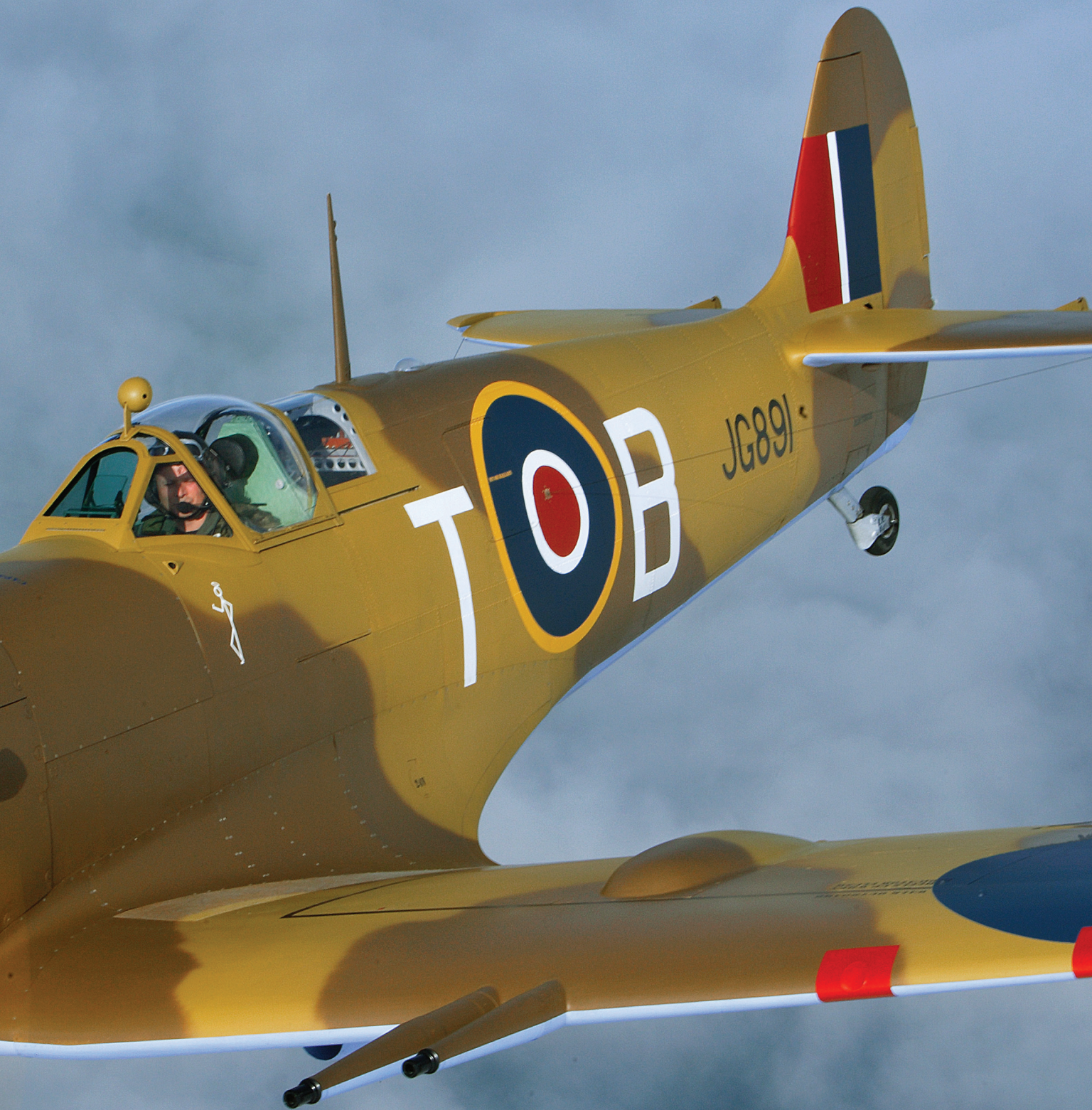
The Spitfire Mk Vc entered service in early 1941, featuring the "universal wing" permitting a variety of armament. Most retained the typical two 20mm cannon and four .303 MGs but some mounted two cannon in each wing. Malta Spits were further modified. Nearly 6,500 were produced into 1943. The prominent chin inlet housed the Vokes carburetor filter for tropical and desert use that reduced top speed by about 10mph and climb rate by 600fpm. (Photo by John Dibbs/planepicture.com)
