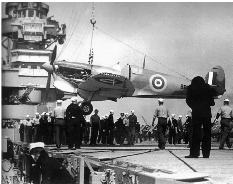
A Spitfire Mk Vc is hoisted aboard the USS Wasp at Port Glasgow, Scotland. The Vc's enlarged air filter, four 20mm cannons and 90 gallon auxiliary fuel tank are visible. The Spitfire's wingtips have been removed to increase space in the carrier's hangar bay.
