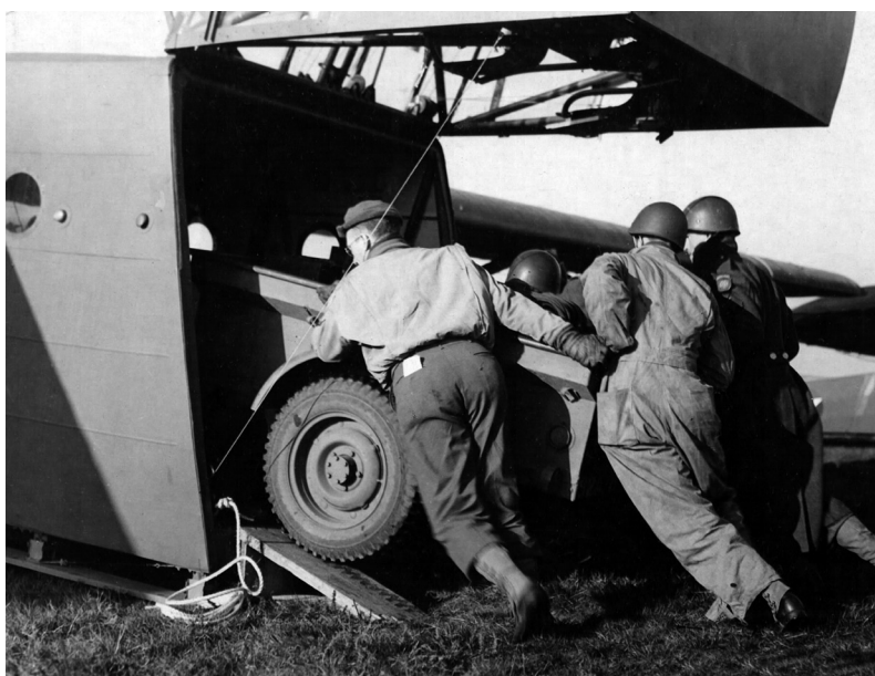
One of the primary design functions of the Waco CG-4A glider was to bring light transport and field artillery to the battlefield. (Photo courtesy of Stan Piet)
