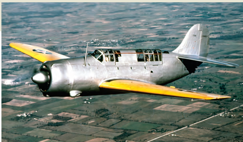
The re-built XSB2C-1 prototype (Bu.Aer. 1758) glides over the Pennsylvania countryside in its attractive pre-war colors. After its R-2600 engine packed up during approach on February 8, 1941, it was repaired and modified with a lengthened fuselage, larger rudder, and an autopilot to deal with its inherent structural and stability vices. Flying again by October 1941, continued flight testing soon revealed further under-design issues when its wing failed during a dive test. The "Beast" was in for a protracted journey to fleet service. (Photo courtesy of Stan Plet)
