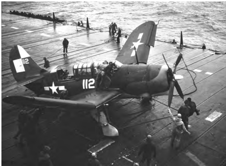
One kinked Curtiss Electric prop blade and a cockeyed parking angle on the carrier deck tell a tale of minor misadventure for this Helldiver. As the wings fold to compress the bomber's footprint, the extended leading edge slats are clearly visible. Somber hues of this color photo are as much as could be resurrected from a magenta-toned wartime Navy image, the bane of some vintage non-Kodachrome film. (Photo by U.S. Navy via Frederick A. Johnsen)
