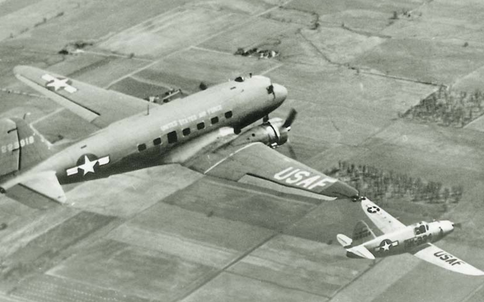
We completed 231 Q-14/C-47 couplings before the switch was made to the EF-84B/ETB-29A aircraft. Note the Q-14's skewed nose angle compared with the C-47's (photos courtesy of author).
