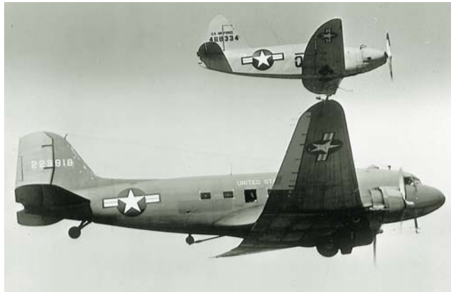
Wingtip vortices and air turbulence initially made wingtip coupling quite tricky, but when I had practiced the procedure, they became less problematic. Seventeen pilots learned to couple the Culver Q-14 to the C-47.
