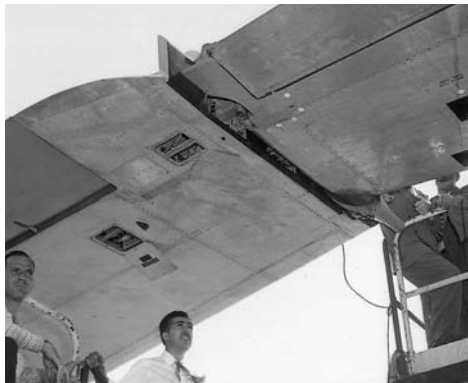
Top: the left-hand EF-84B's right wing lance is in position to contact the EB-29A's left wing receiver. Center: once contact had been made, the receiver retracted into the EB-29A's wing and the planes were fully coupled. Above: fitted to the EB-29A's wingtip was a rubber seal, so when the wingtips were in the retracted position, there was an airtight bond between them.
