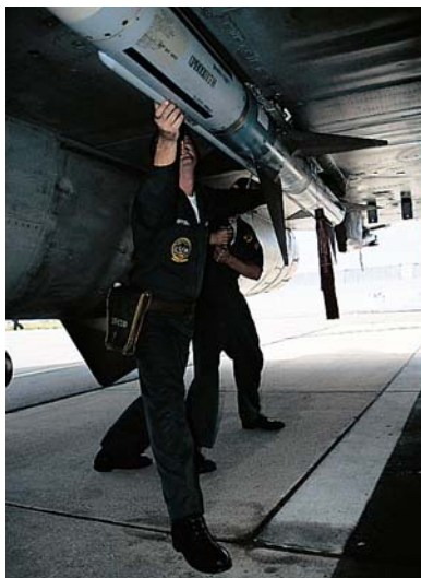
When attached to the launcher, two of the missile's 16-inch-wide triangular fins protrude into the bottom of the fuselage (photo by Ted Carlson).
