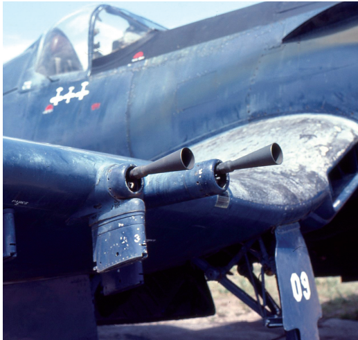
Honduran F4U-5s retained their original armament of four 20mm cannon, nominally with 230 rounds per gun. This is Soto's No. 609 that knocked down a Mustang and two Corsairs. (Photo by Dan Hagedorn)
