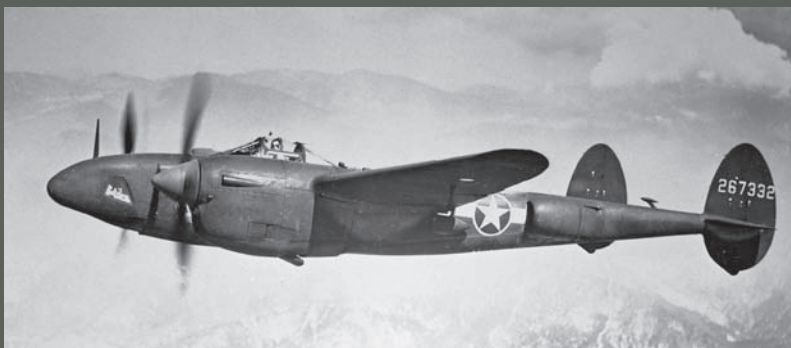
Lockheed F-5B photo Lightning shows evidence of synthetic haze paint under the wing, where lighter top coat was applied more heavily than on upper surfaces. Radio mast on top of nose, lack of gun barrels, and flattened lower nose surface help identify this as a photo Lightning. (Photo courtesy of Lin Hendrix collection via SDAM)
