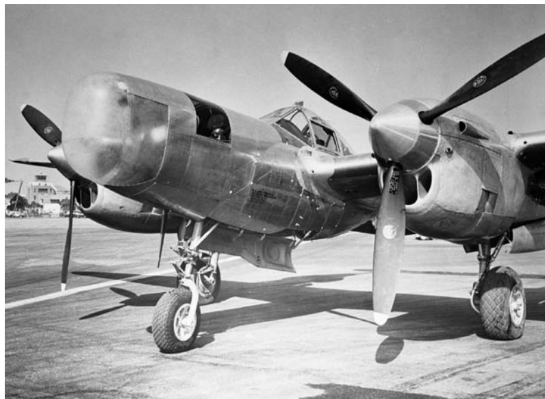
Translucent nose on a Pathfinder P-38J (44-23139) accommodated radar. (Photo courtesy of Lockheed)
