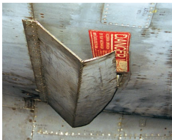
Dive flaps altered airflow at high speeds, giving the P-38 pilot a way out of compressibility problems. (Photo by Frederick A. Johnsen/AIRAILIMAGES)
