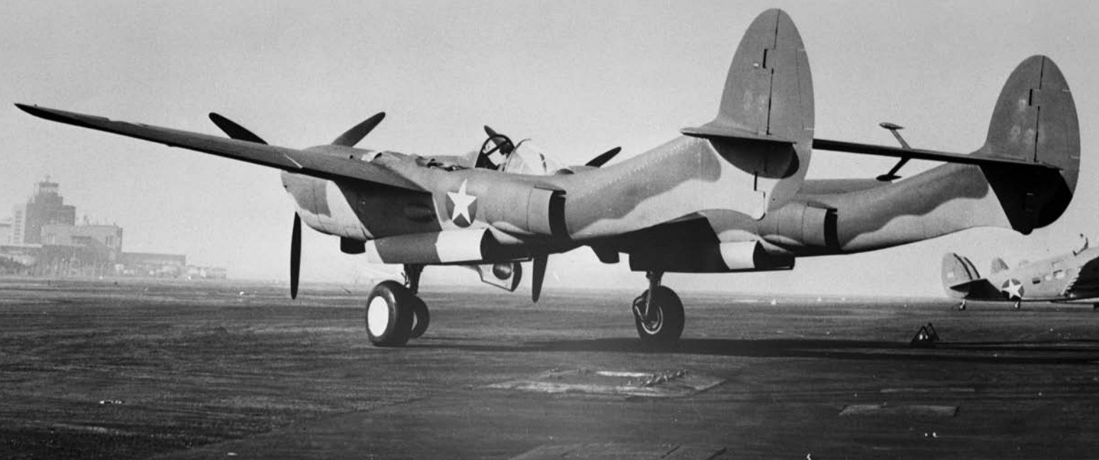
P-38 upswept tail booms photographed in December 1942 explored high-speed flight issues. (Photo courtesy of Lockheed)
