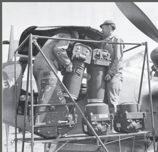
Fresh K-17 cameras are loaded into F-5A 42-12778 Dim View assigned to Lt. Walter D. "Dale" Shade of the 13th Photo Recon Sq, 7th PRG. (Photo courtesy of Stan Piet)
