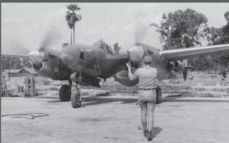
F-5G Lightning Miss Virginia G of the 21st Photo Recon Sqd. taxis out of its hardstand prior to mission during 1944. The paint has been removed from the spinners and the leading edges of both wings to save weight and decrease drag in order to increase Lightning's speed. (Photo courtesy of Jack Cook)
